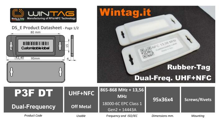
Flexible Rubber RFID Tag, Dual-Frequency P3F Series. UHF + NFC double-frequency RFID transponder, made of TPE rubber very resistant outdoor and aggressive chemicals, OFF Metal use. Inside there are 2 distinct UHF + NFC tags that can have the same electronic coding
